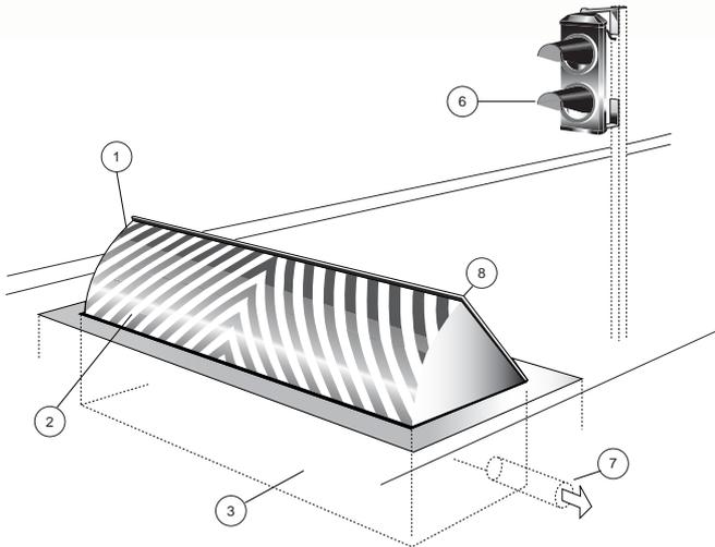
The hydraulic road blocker RSB76H was designed as an effective means of controlling access to high security areas (Impact resistance: theoretical K4 - 610KJ) such as embassies, airports, strategic factory sites, etc ...The RSB76H offers the advantage of not requiring a side column to house the drive mechanism.
